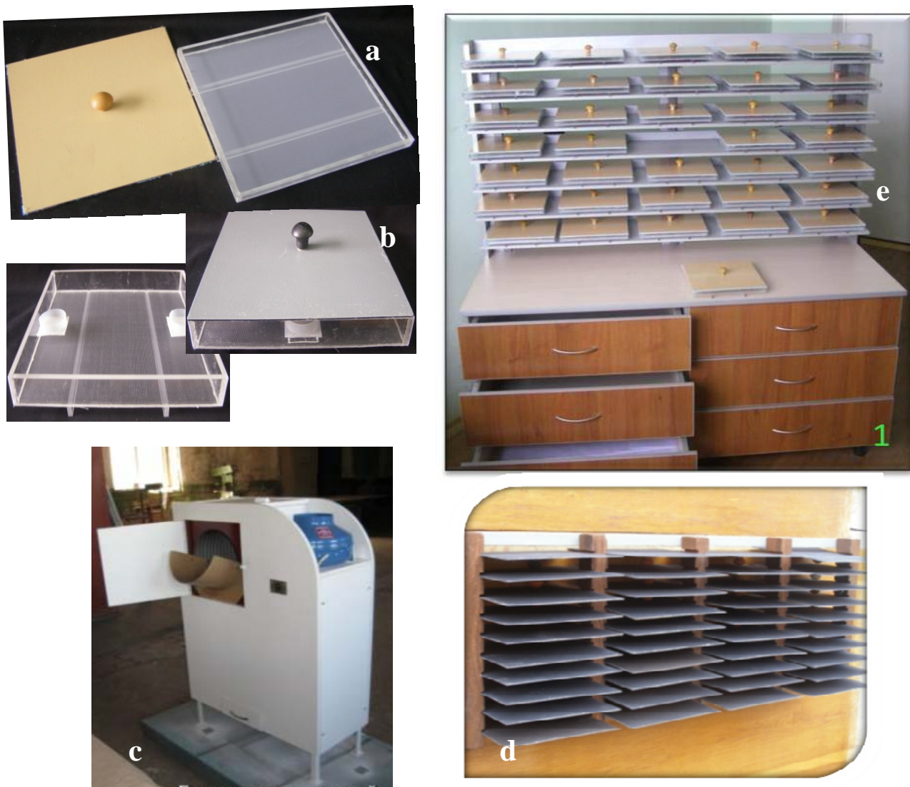
Fig. 3 The equipment for the production of the common green lacewing.
