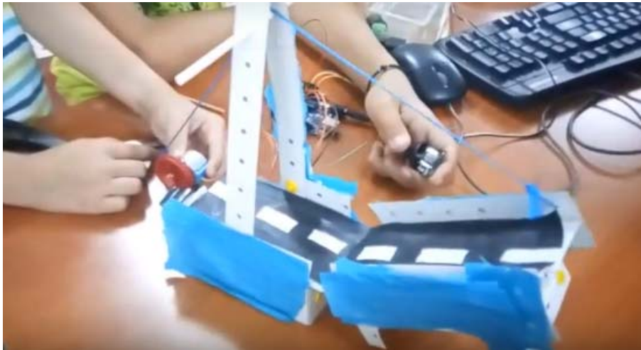
Figure 2. Bridge lifted by a mechanism using Arduino.
