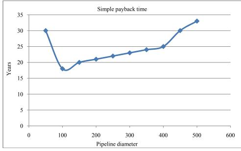
Fig. 6 Simple playback time of outlays for replacement of a DH system.
