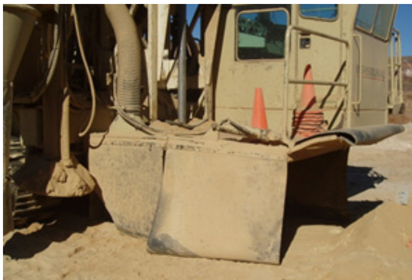
Fig. 6 Open slits between rubber belts of the shroud.
