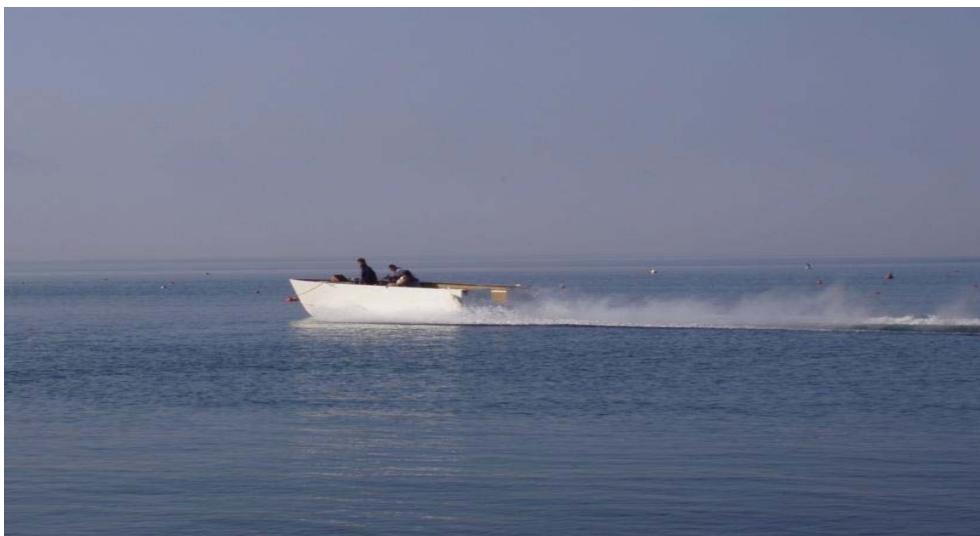
Fig. 3 Self-propelled model hull navigating on Bolsena Lake (speed 22-24 knots).
