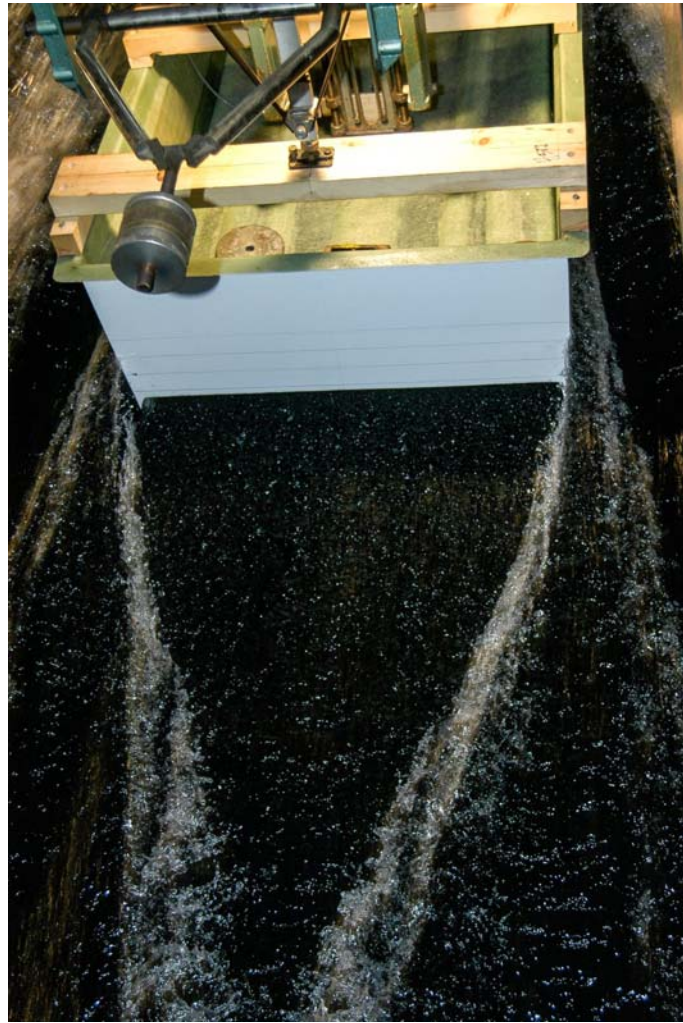
Fig. 7 Spray hull Test towing \Delta 70t - speed 24 knots, Towing Tank INSEAN CNR Rome, 2010.
