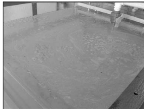
Fig. 8 Photograph of oily foam formed on free surface of flotation chamber prior to implementation of level control strategy.
