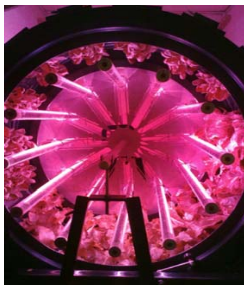
Fig. 1 Lettuce in the rotary system rotates around the 12 LED tubes held by a support structure.
