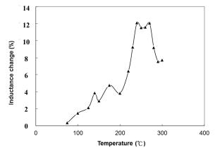
Fig. 8 The inductance shift of chip samples after thermal treatment with different peak temperatures.
