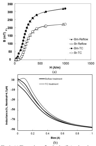
Fig. 6 (a) The maximum flux density (Bm) and maximum remanence (Br) of before- and after-treatment of circular type samples; (b) the L-I curve of before- and after-treatment of chip type samples.
