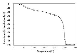
Fig. 9 The temperature characteristic of the inductance trend of chip samples.
