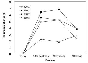
Fig. 11 The inductance shift trend of chip samples which were cooled from different peak temperatures.
