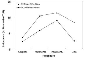
Fig. 7 The inductance shift of chip samples after two different thermal treatments in series.
