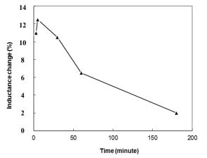
Fig. 10 The level of inductance of chip samples treated at 270 °C with different soaking times.
