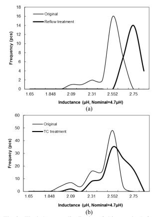
Fig. 2 The inductance distribution of chip samples before and after treatments, (a) reflow treatment, and (b) TC treatment.
