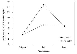
Fig. 12 The inductance shift of chip samples undergoing thermal cycling with different peak temperatures.
