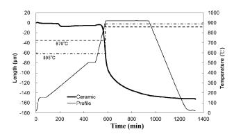
Fig. 4 The TMA of NiCuZn ferrite material.
