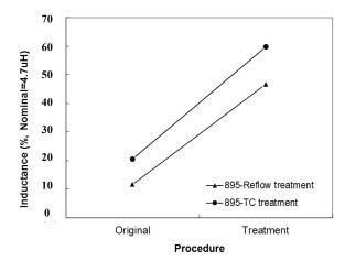
Fig. 3 The inductance shift of chip samples firing at 895 °C.
