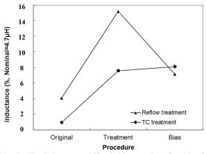
Fig. 5 The inductance shift of chip samples after bias for each treatment.
