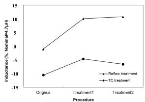
Fig. 1 The inductance shift of chip samples after two treatments in series.
