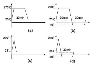
Fig. 13 The treatment profiles of chip samples to see the role of subzero temperature; (a) without the subzero temperature stage, (b) with the subzero temperature stage, (c) without soaking time at the peak temperature and without the subzero temperature stage, and (d) without soaking time at the peak temperature and with the subzero temperature stage.
