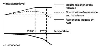
Fig. 15 The inductance change caused by the stress-release and remanence.
