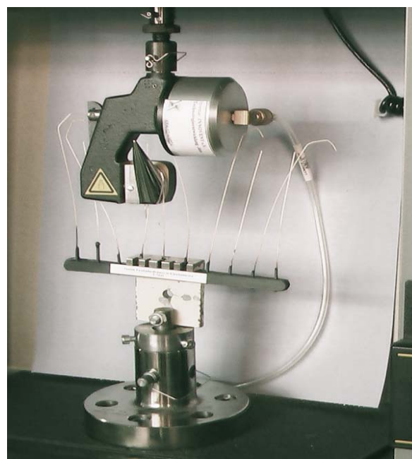
Fig. 1 Experimental setup of testing the maximal thread pullout-strength (T-test).
