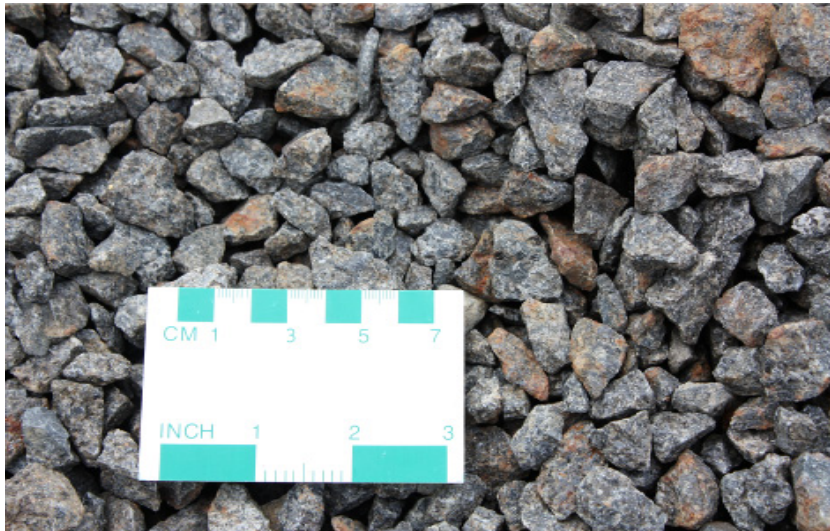
Fig. 3 Crushed coarse aggregate (anorthositic gabbro).
