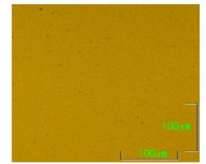
Fig. 4 Microstructure of polymer-rubber modified bitumen (CR) after 180 °C temperature conditioning measured on the bottom of cylinder after 7 days.
