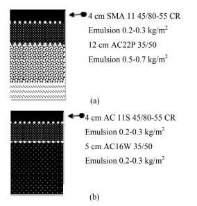
Fig. 5 Trial sections containing polymer-rubber modified bitumen 45/80-55 CR: (a) wearing coarse SMA 11; (b) wearing coarse asphalt concrete AC 11.
