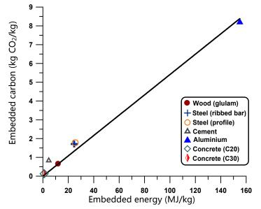
Fig. 2 The relationship between embedded carbon and embedded energy.
