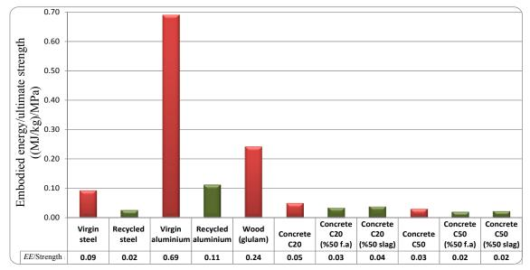
Fig. 5 Embodied energy to strength ratios in structural materials.
