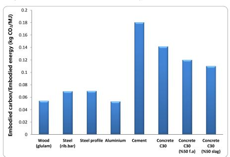
Fig. 3 Embodied carbon to embodied energy ratios in structural materials.
