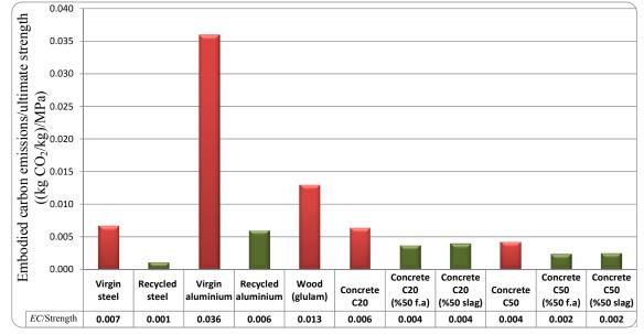
Fig. 4 Embodied carbon emissions to strength ratios in structural materials.
