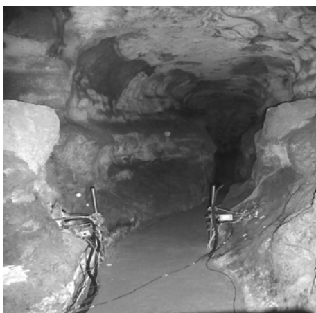
Fig. 9 Microclimatic instruments installed in the so-called Painted Gallery of the Lascaux Caves, France.
