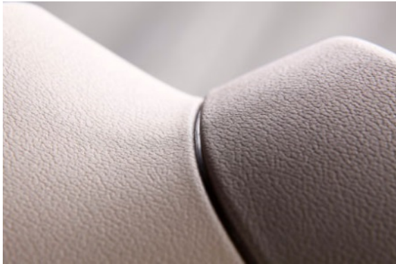
Fig. 1 Example for a molded skin produced by slush molding for interior panels in cars [1].
