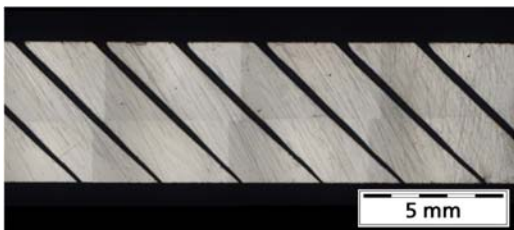
Fig. 7 Longitudinal section of holes drilled into 5 mm thick material with an angle of 45°. The holes are drilled from the upper side.
